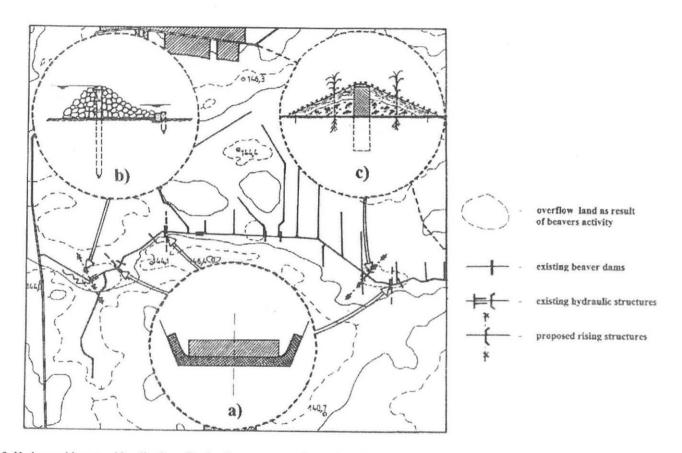
ig. 3. Hydrographic net and localisation of hydraulic structures at the section of the Małynka river valley predicted for restoration: a) gabion step, b) dam constructed from wood and stone covering, c) "camouflage of concrete gate
