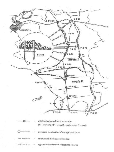
Fig. 2. The Sumiackie Meadows - hydrography, existing hydrotechnical structures and proposed technical solutions
