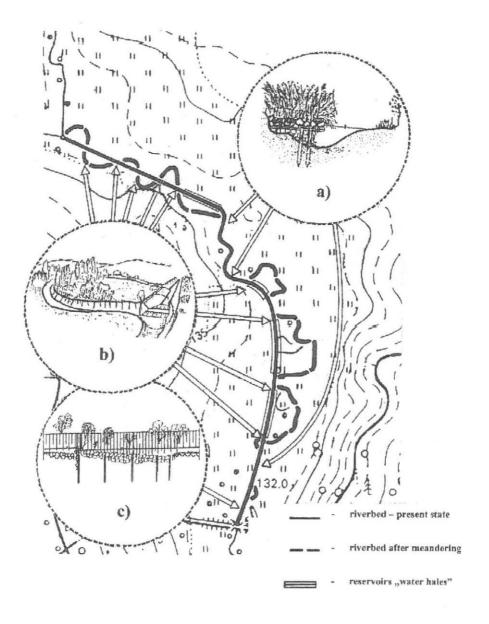
Fig. 1. The Rudnia's river valley segment of intendent for restoration, technical activities proposed: a) riverbed narrowing structures, b) dykes affecting water flow by meanders, c) stone spillway
